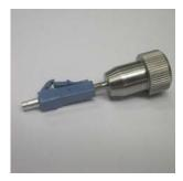
Insert the tool into LC ferrule, press and rotate 60 degrees then test .
